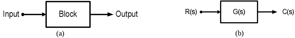
Fig.5.1. (a) A block diagram representation of a system and (b) A block diagram representation with gain of a system
