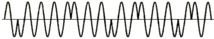
Section of biphase modulated spread spectrum ultrasonic waveform
