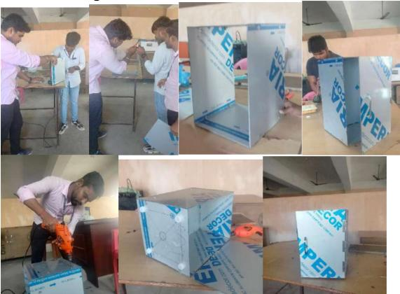
By v shape corner joint. Nut and bolt .washer . Door handle and door connector door locker and Leg we successfully make frame of refrigerator
