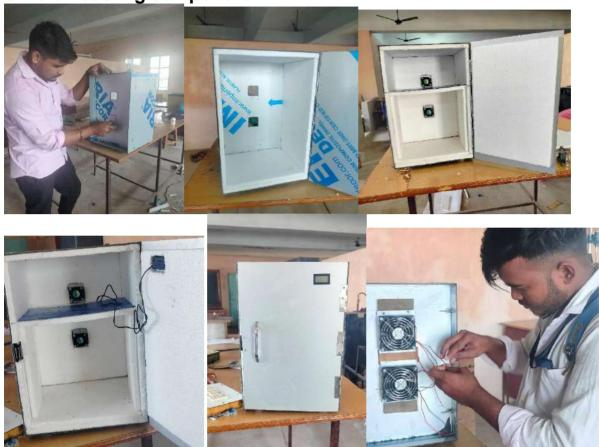
Install cooling component backside of the refrigerator and install a digital thermometer front of the refrigerator
