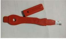
We cut (1×1) foot 2 and (1.5×1) foot 4 sheet for Frame making. We use PVC cutter for cutting
