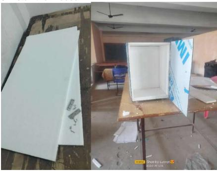
• We install thermocoal inside the refrigerator for keep the temperature
