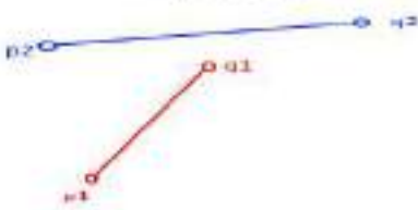
Example: Orientations of (p1,q1,p2) and (p1,q1,q2) are different. Orientations of (p2,q2,p1) and (p2,q2,q1) are same.
